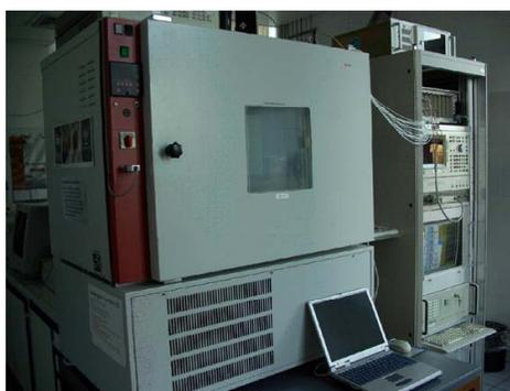
Figure 3: Test gas mixture system and test chamber (GASI)
